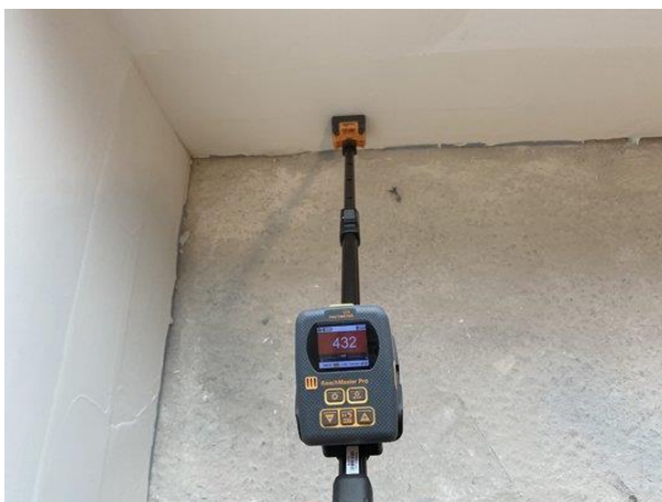
Typical local EMC in areas with heavy coats of spackle
